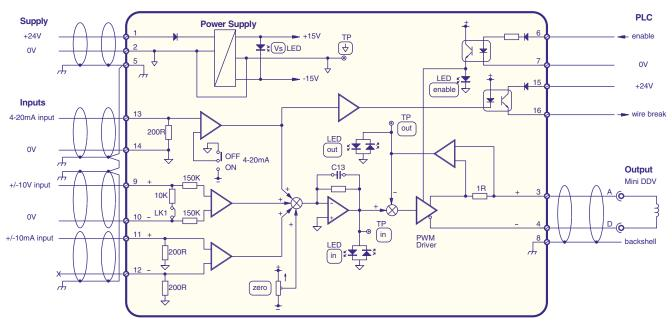
\* note: LK1 is a cuttable link on the solder side of the PCB.
